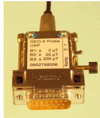
probe plug UAP ± 70 µT compensation can be additionally activated
