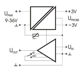
The AS-probe adapter is designed for autonomous operation of our AS-active probes without teslameter.
