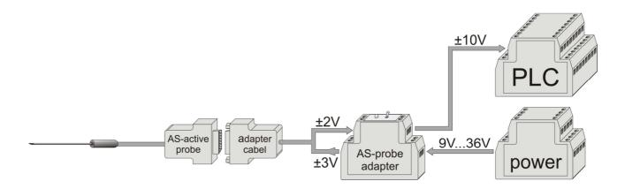
The analog output of the adapter is calibrated and thus can be used e.g. for displaying magnetic pulses in the µs-range (oscilloscope), recording of measurements and for field control. The bandwidth of the analog output reaches from DC to a least 100 kHz. Therefore it is suitable for measuring both constant magnetic fields and alternating magnetic fields. The actual usable bandwidth depends on used AS-active probe.
